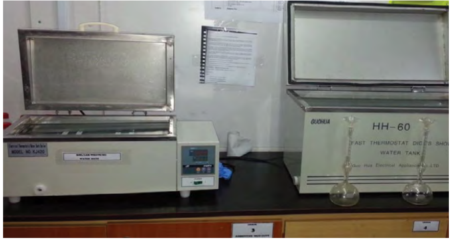
WATERBATHS AND Le CHATELIER'S FLASKS FOR BARITE ANALYSIS
